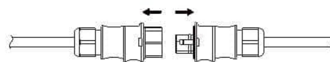
3. Cover the PV module with an opaque, and then disconnect the PV module DC connectors from the microinverter.
