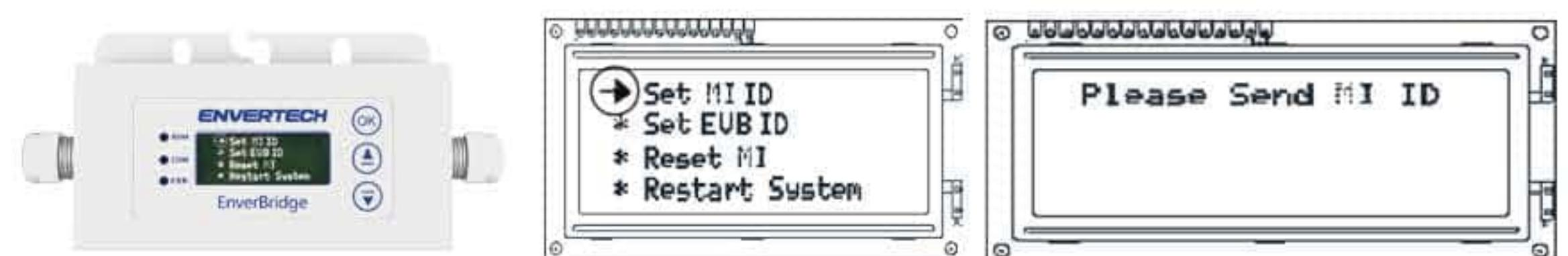
4) Then you can press "Send" button in the software to complete the setting. Meanwhile, "ID Set OK" will be also shown on the EVB202 screen. Thus the MI binding process is completed.
